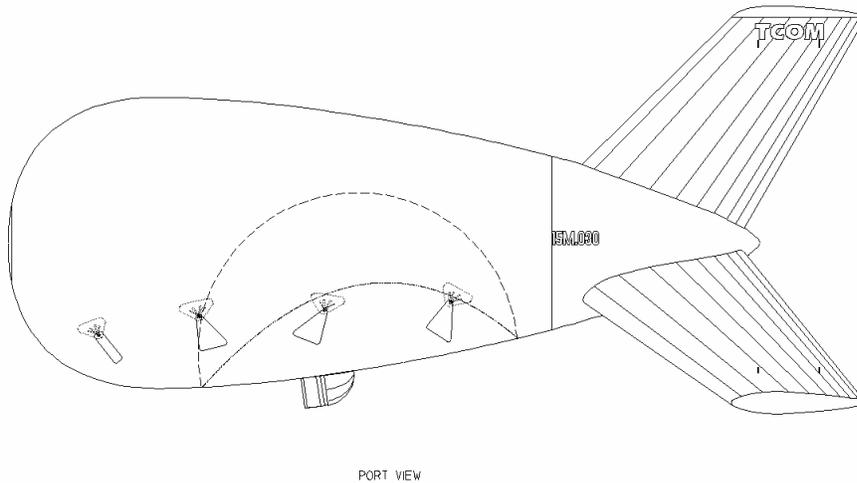
**Figure 1. 15M® Aerostat Flexible Structure**
