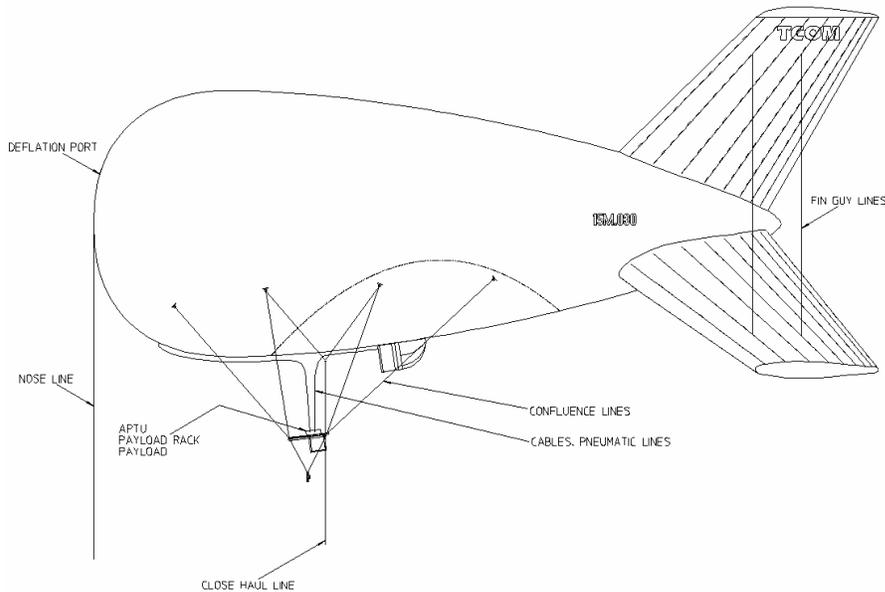
**Figure 2. 15M® Aerostat Installation**
