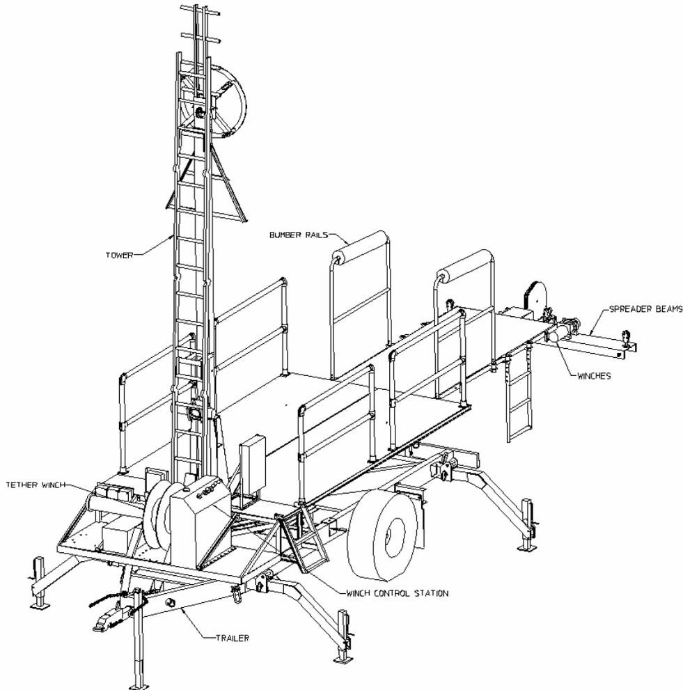
**Figure 3. Mooring System Deployed**
