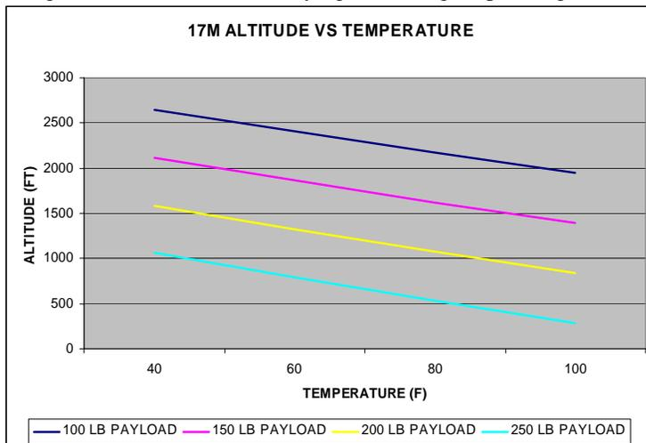
**Figure 11. 17M Altitude vs. Temperature**
