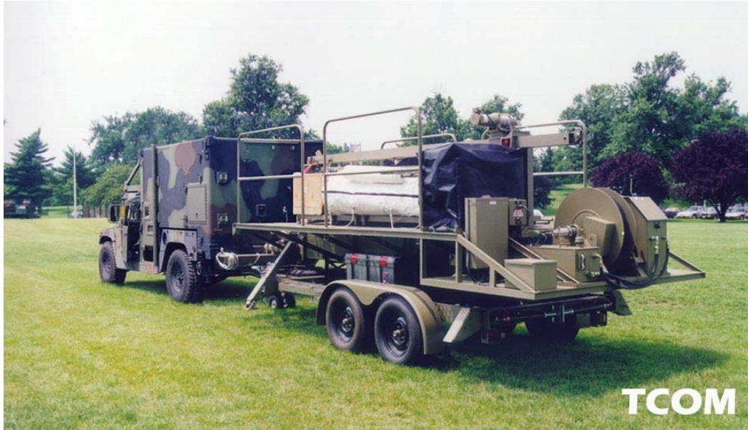
Figure 4. Mooring System Packed
