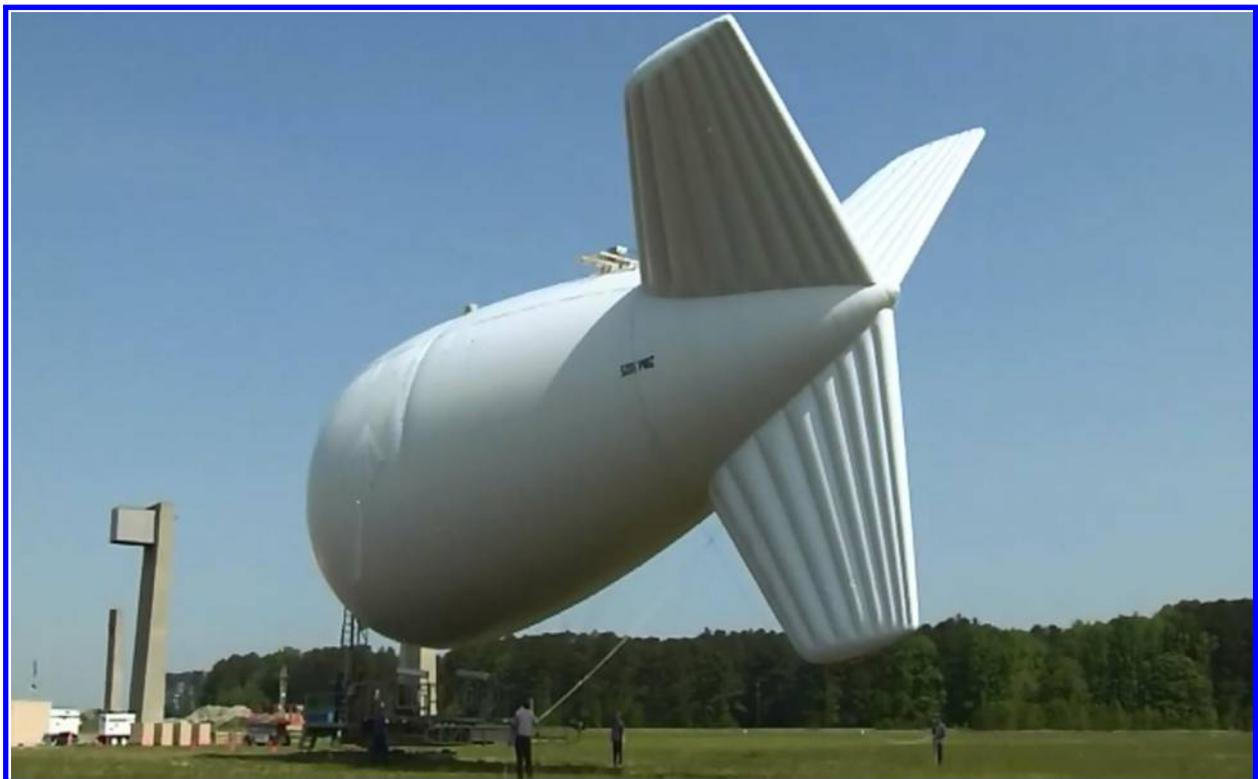
**Figure 10. Aerostat Rolled Upside Down For Maintenance**
