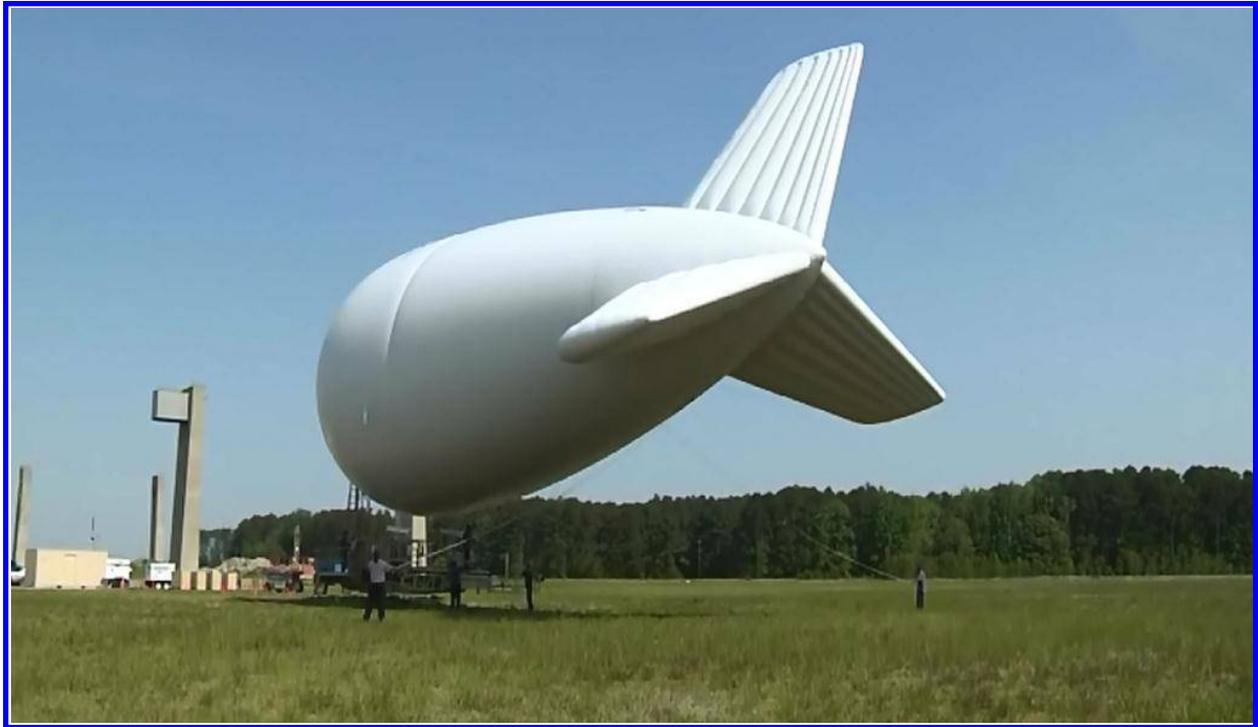
**Figure 9. Aerostat Rolled To Side For Maintenance**
