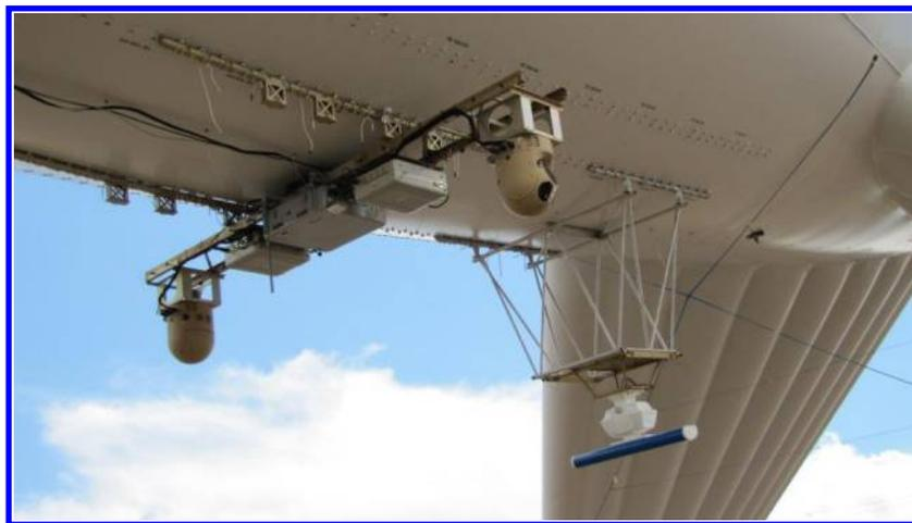
**Figure 6. Payload Racks**
