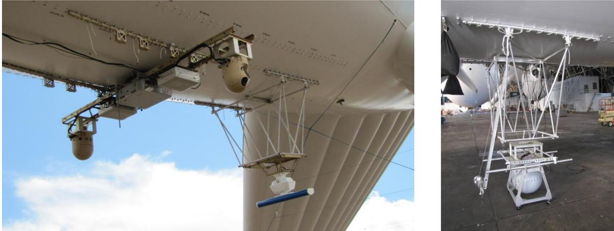
**Figure 6. Payload Racks**
