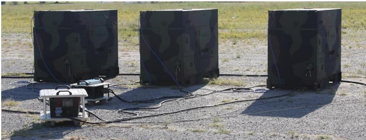
**Figure 7. Power Generators Connected in Parallel**
